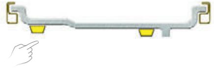
Rim cutaway displays selected weight mode
