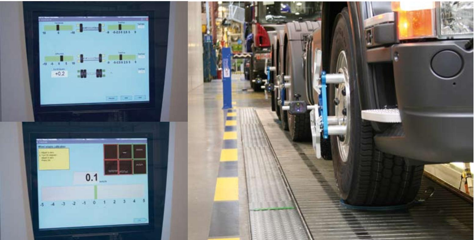
The system can be configured for all vehicle types with their different axle configurations, and target values as well as tolerances can be entered into the software. The adjustments can only be finished when all values are in tolerance. This ensures that every vehicle that leaves the production line is properly aligned.
