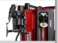
This mounting tool guides the tyre during the mounting procedure, and assisted by the bead pusher the upper bead breaker disc presses the tyre most gently into the drop centre of the rim.
