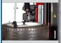
The integrated demounting lever levers the upper tyre bead over the rim flange – absolutely preserving to both tyre and rim. Finally the lower bead is demounted automatically by means of the demounting tool.
