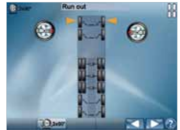
2 measuring heads mode Quick measurement of front axle
