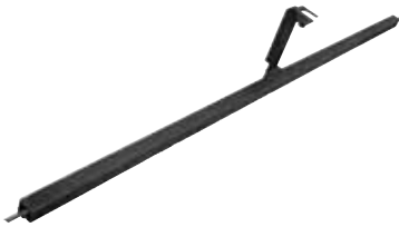
Adaptor rod for semitrailers' king pin
