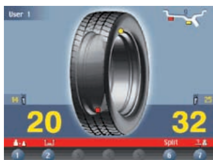
RPR function (Rear Planes Residual). It allows the simultaneous visualization of unbalance values: at the set correction planes, at the real correction planes (clip-on weight on rim edges).
