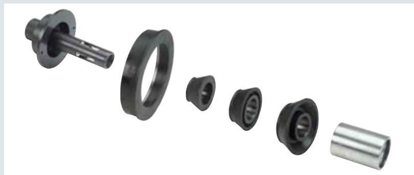
UC202/SE pneumatic cone adaptor 65mm Ø shaft with 3 cones, for light truck wheels having central hole Ø 76 to Ø 178 mm.
