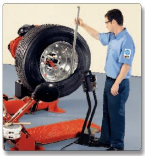
The standard hook tool is used to mount and demount tubed and super single tires or more difficult-to-handle wheel assemblies.
