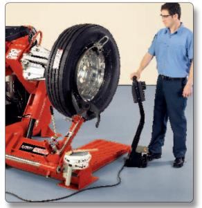
Position the wheel pliers and roll the first bead onto the rim. Reposition the pliers and roll the second bead on. It's that easy!
