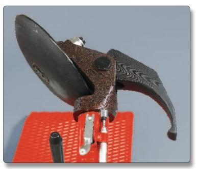
Tool head includes standard disk and hook for bead loosening, mounting and demounting tires. The hook tool folds out of the way when not in use. Standard and optional tool heads are quickly and easily changed out.
