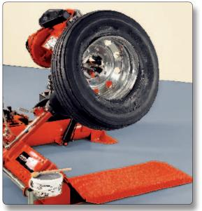
Bead loosening and demounting can be as easy as rolling the tire off of the rim in a single step.
